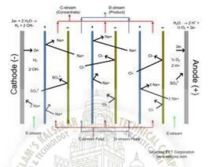
For more efficient separation, ion selective membranes, which are permeable to only one kind of ions with specific charge, have been used in recent years.
