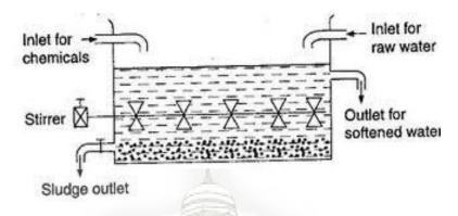
It consists of a tank provided with inlets for raw water and chemicals, outlets for softened water and sludge, and a mechanical stirrer for thorough mixing.
