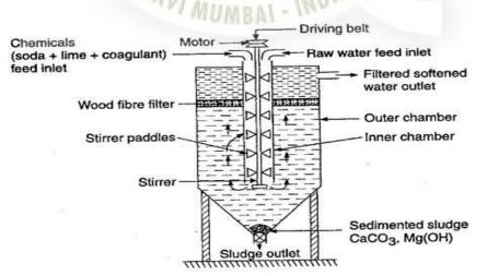
It consists of an inlet for raw water and chemicals, and outlet for softened water and sludge; and a rotating shaft having paddles.
