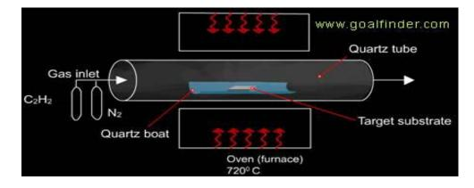
In this process a mixture of hydrocarbon gas (ethylene ,methane or acetylene ) and a process gas (ammonia ,Nitrogen, hydrogen) is made to react in a reaction chamber on heated metal substrate to a temperature of around 700°c-900°c at atmospheric pressure.
