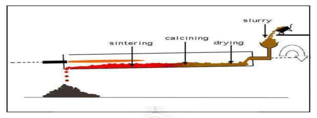
It is carried out in rotary kiln which is a steel tube of about 2.5 to 3.0 m in diameter. and 90 to 120 m in length, lined inside with refractory bricks.
