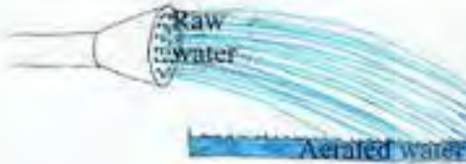
Spray Nozzle Aerator
