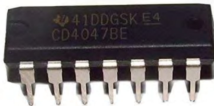
Fig. 12. CMOS low power multivibrator.
