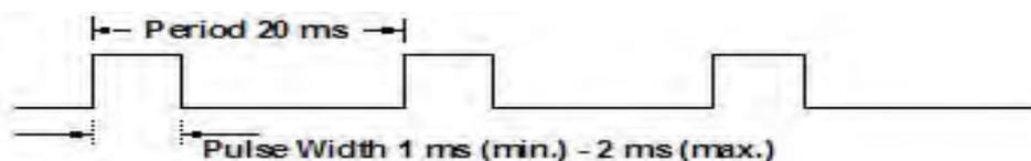
The angle is determined by the duration of a pulse that is applied to the control wire. This is called Pulse width Modulation. The servo expects to see a pulse every 20 ms. The length of the pulse will determine how far
