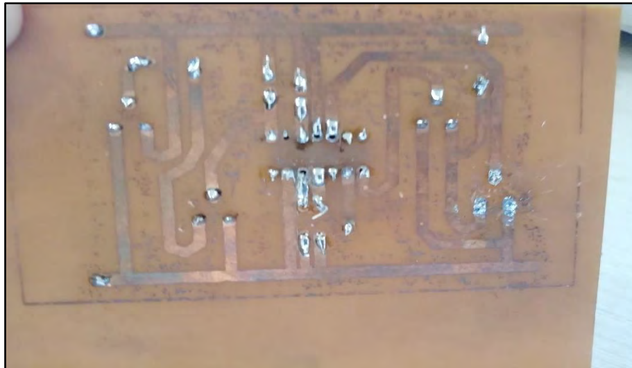
Fig. 6.6 Soldering of Tone Generator PCB
