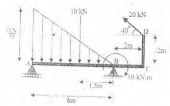
Determine the moment to be applied at C for equilibrium of pin jointed mechanism. Use virtual work method. Refer Fig. (06)
