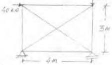
(b) Work out the vertical deflection of point C due to change in temperature as 07 indicated. Take thickness of each member 400 mm, and  $\alpha_1 = 12 \times 10^{-6} e^{-6} C$ E=200 GPa
