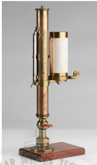
Figure 2.3: McNaught Steam Engine Indicator (Replica).
