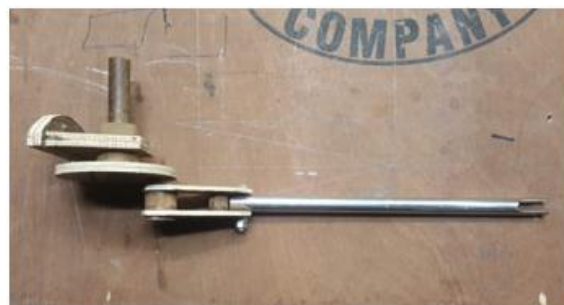
Figure 5.4: Piston Rod for Connecting Cylinder with Indicator Drum.
