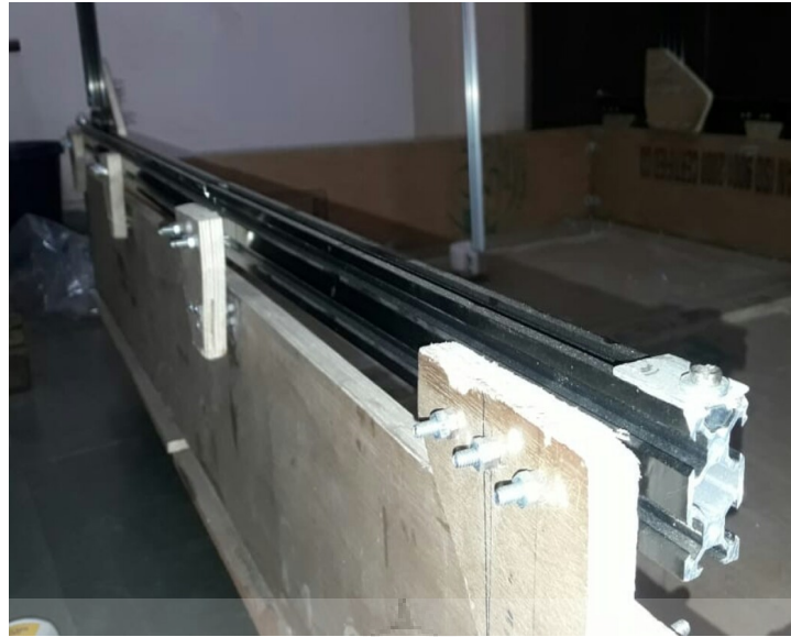
Figure 4.35: Placing of Aluminum Extrusions
