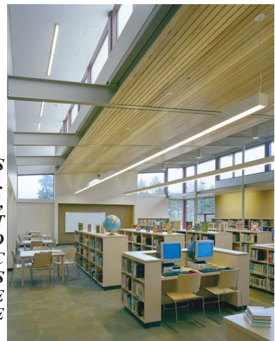
C5.FIG.10 THE LIBRARY, WHICH UTILIZES CLERESTORY WINDOWS FOR DIFFUSE DAYLIGHTING.
