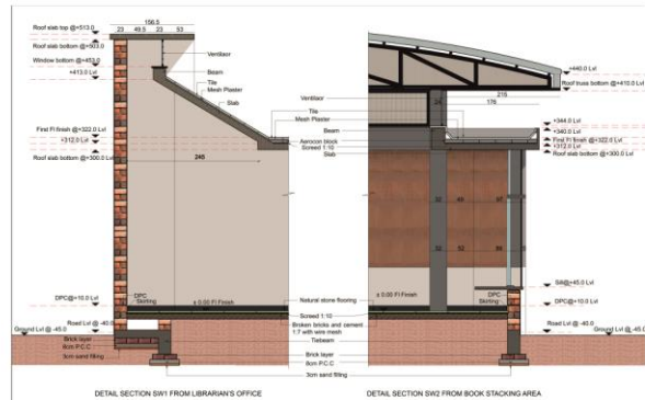
C2 Figure No:03 CONSTRUCTION DETAIL
