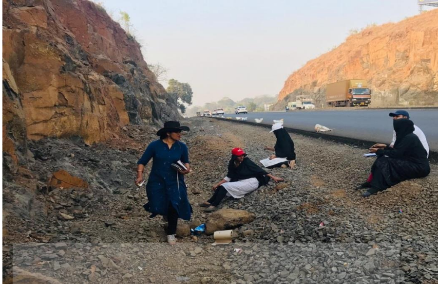
Fig. 3.1 Compact Basalt exposed in the study area is altered by weathering along the joints
