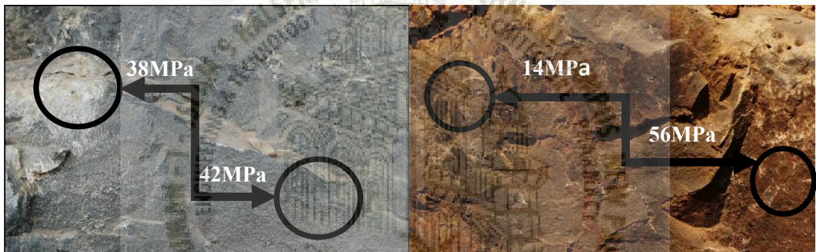
Fig. 3.12 Schmidt Hammer tests at the field
