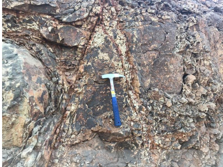
Fig. 3.3 Joint set J1 trending NE-SW and J2 trending NW-SE
