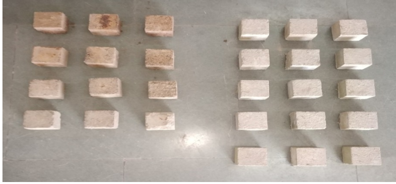
Fig 4.1 Pictorial view of Cement-POP & Cement-Bentonite cubes
