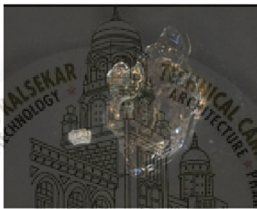
Figure 1.2. Dry and swollen SAP particle (figure with courtesy of BASF) (Source: Viktor Mechtcherine mechtcherine@tu-dresden.de, Hans-Wolf Reinhardt reinhardt@iwb.uni-stuttgart.de, DOI 10.1007/978-94-007-2733-5)
