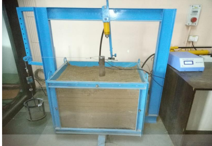
Fig 3.2 Experimental setup of Single pile
