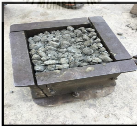
Figure 2.2 Casting of Cubes
