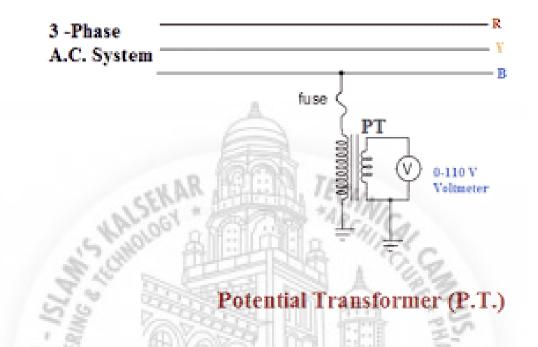
Potential transformer is a voltage step-down transformer which reduces the voltage of a high voltage circuit to a lower level for the purpose of measurement. These are connected across or parallel to the line which is to be monitored
