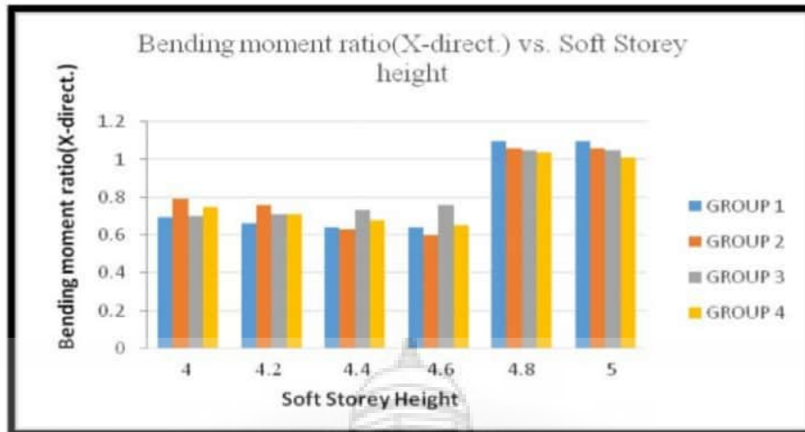
Graph 4.20: Variations of Bending moment(X-direct.) for different soft storey heights and column groups
