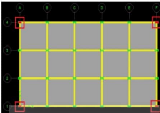
Figure 4.3: Group 1 (Corner exterior columns)
