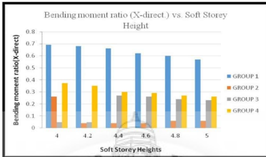
Graph 4.5: Variations of Bending moment(X-direct.) for different soft storey heights and column groups
