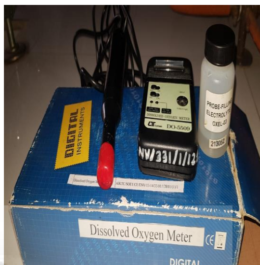
Figure 3.2: DO Test (It is used to determine the amount of oxygen present in the sample before and after treatment)
