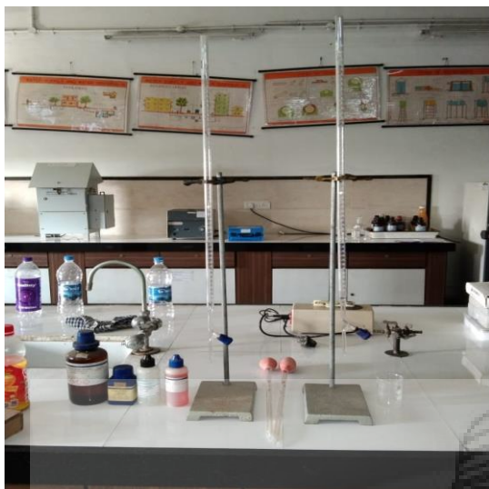
Figure 3.1: Hardness Test (Apparatus to determine hardness present in sample by titration with EDTA until changes colour from pink to colourless)
