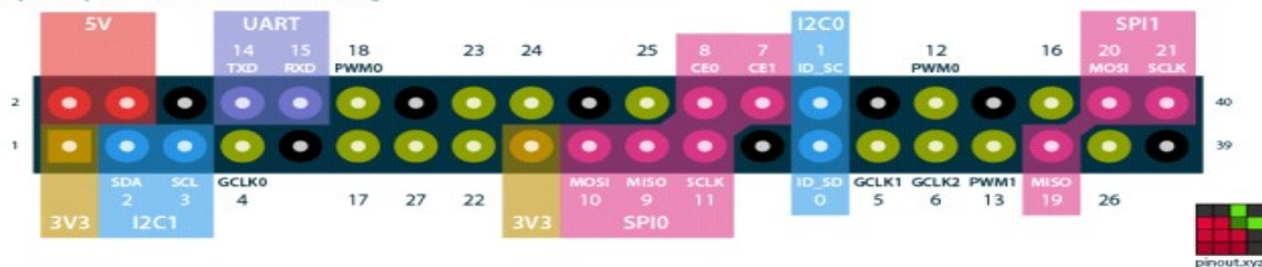
Raspberry Pi GPIO BCM numbering
