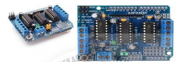
L293D use 16 pin DIP package, its internal integration is bipolar H - bridge circuit. This kind of bipolar pulse width method has many advantages, such as the current continuous, or microcurrent vibration when the motor stops, which as a lubrication effect. It can eliminate the dead zone of static friction when positive and negative
