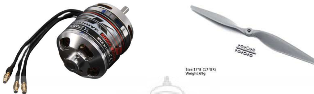
Figure 3.4 - Turnigy Sk3 5055-430kv and 17x8 APC style propeller.
