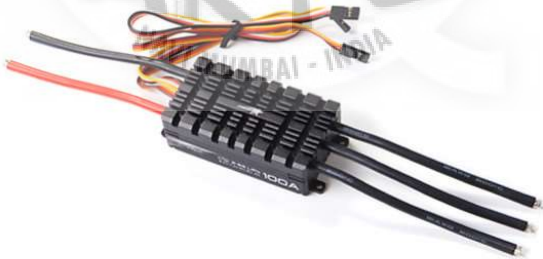
Figure 6.5 - AeroStar WiFi 100A Brushless ESC with 5A BEC. [26]
