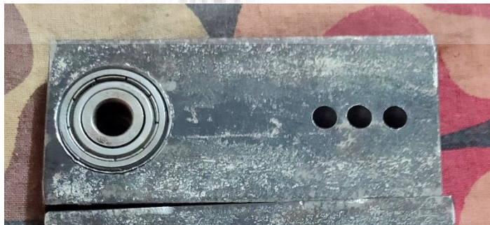
Figure 5.2.5 Side plate with Bearing
