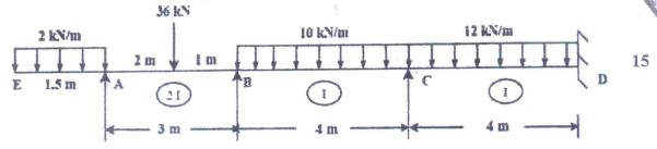
Q.3 (a) Find the Plastic Moment 'Mp' for the continuous beam given below.
