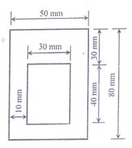
(b) Both machine components AC and PS are acted upon by a tensile load of 50 kN. Find the ratio of their strain energies. Take E = 2E5 N/mm<sup>2</sup>.
