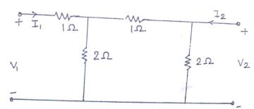
Q6. (a) Determine voltage transfer function  $V_2/V_1$  for given network.
