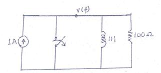
(b) In the network shown in figure the switch is closed and steady state is attained. At at t=0, switch is opened. Determine the current through the inductor.
