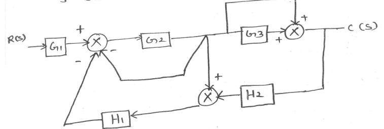
a) consulate T.F. for following SFG by using mason's Gain formula.
