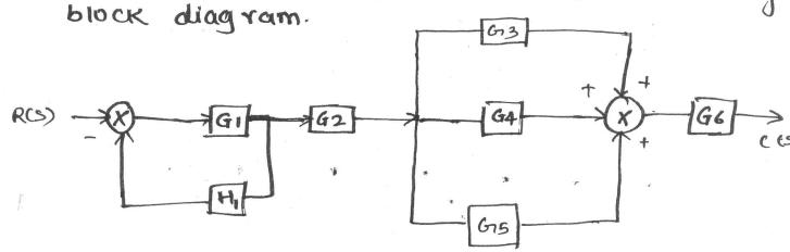
solve are one out of Two (10)out the transfer of given diagram Find by using Block reduction method.
