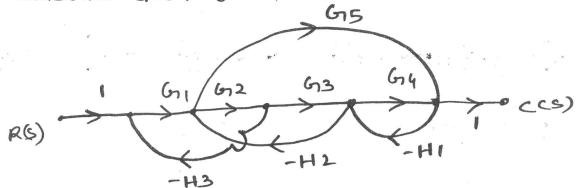
b) calculate T.F. 50% Following SFG by using Manson's Gain Formula.
