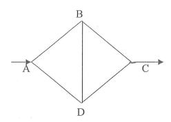
Where K=1 for AB and CD , K=2 for BC and AD, K=3 for BD and Input at A is 30 units and output at C is 30 units
