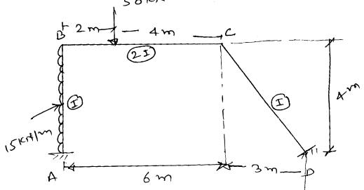
4. (a) Analyse the pin-jointed structure shown in **figure** by flexibility method the cross 12 sectional area of each member is 20 cm<sup>2</sup>. Take E = 2000 kN/cm<sup>2</sup>.
