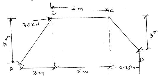
3. Analyse the frame as shown in **figure** by method of moment distribution and draw **20** B.M.D. (length AB = 4 m).
