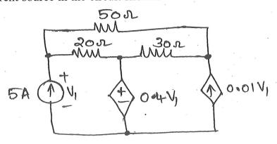
6. (a) Find the Thevenin equivalent of the network shown. What power would be delivered to a load of  $100 \Omega$  at a and b?
