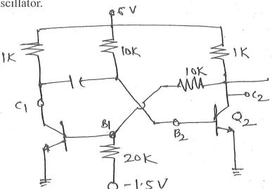
For the above circuit, compute voltage levels and sketch the waveform of voltages at  $B_1$ ,  $C_1$ ,  $B_2$  and  $C_2$  for permanant state and quasi Stable state.
