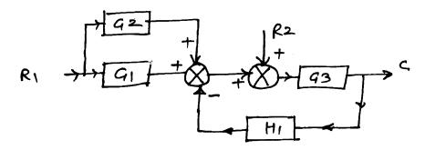
(b) Find the transfer function of the following system by using signal flow graph. 10
